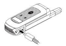
3. Insert the other end of the data cable into the data port of the other device.
